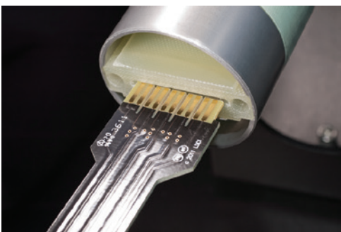
Sliding a sample card into the insert
